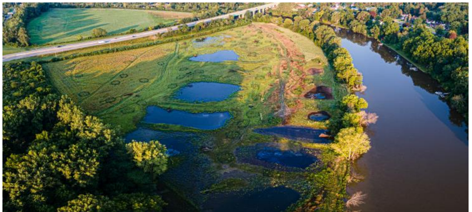
Large wetland pools separated by seepage berms along the Sandusky River at Redhorse Bend Preserve.
